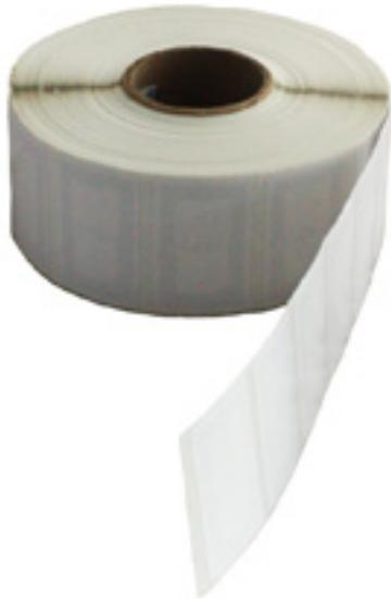
The MIFARE Ultralight C chip from NXP, in a card-sized label format. Operates at 13.56 MHz wireless frequency, according to the ISO 14443A standard. This chip operates a MIFARE Ultralight compatible command set and contains 144 bytes of usable read/write memory with secure data access and cloning protection via 3DES authentication.
